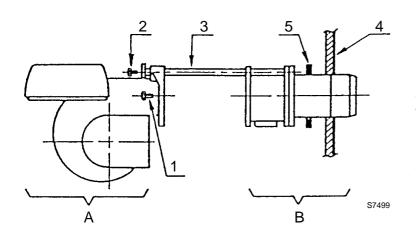
Separate the combustion head from the burner body by loosening the screws 1) and 2) and withdrawing the group A) from the holding bars 3).
