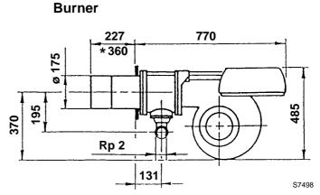
\*Length available with special blast tube to be separately required.
