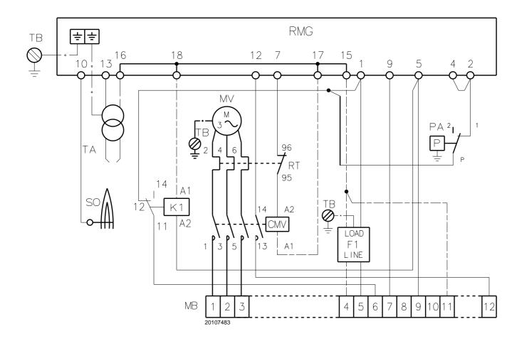
CMV Fan motor contactor
