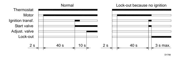
If during operation the flame shuts off, lock-out occurs within 1 sec.
