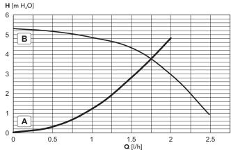
A = Boiler pressure losses - 1,2 e 3 = Circulating pump speed
