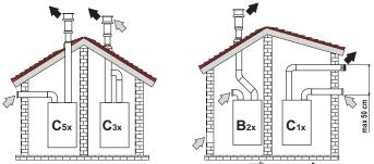
fig. 17 - Examples of connection with separate pipes ( = Air / ==
