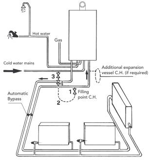
fig. 9 - Automatic bypass connection
