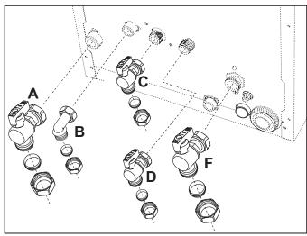
fig. 10 - Isolation valve kit
