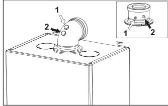
fig. 26 - Flue gas sampling point
