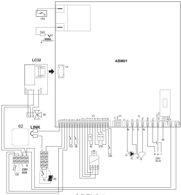
fig. 34 - Wiring diagram
