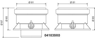
fig. 18 - Starting accessory for separate ducts
