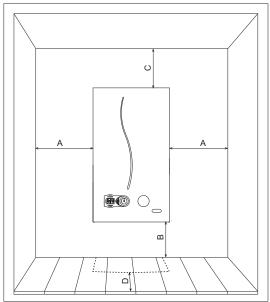
fig. 8 - Minimum distances around the boiler
