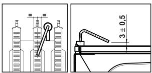
fig. 25 - Electrode positioning
