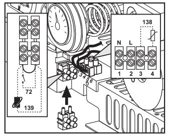
fig. 12 - Accessing the terminal block
