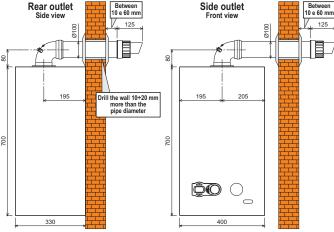
fig. 14 - Standard coaxial installation
