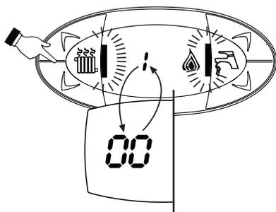
fig. 14 - TEST mode (heating power = 100%)
