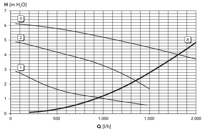
A = Boiler pressure losses - 1, 2 and 3 = Circulating pump speed
