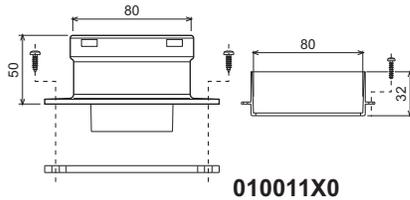
fig. 12 - Starting accessory for separate ducts
