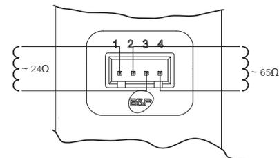
fig. 16 - Gas valve connection
