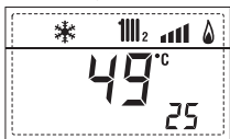
26. Display safety thermostat with board MIXED ZONE 2 (input S1) respectively ON and OFF
