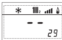
30. Display solar probe temperature value S1 with SOLAR board
