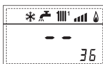
45. Visualization temperature heating refers to the third circuit
