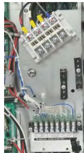
Close-up view of terminal block sub-assembly
