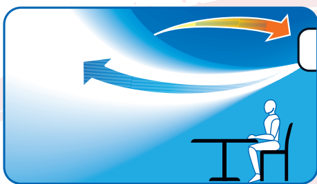
Correct louvre positioning ensures draught-free comfort
