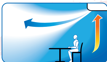
Under-ceiling units allow louvre adjustment so that the air flow is guided along the ceiling above the room occupants.
