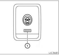
The dynamic driver assistance switch is used to temporarily activate the Intelligent Lane Intervention (I-LI) system that is enabled using the settings menu of the vehicle information display.
