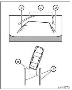
3. Slowly back up the vehicle adjusting the steering wheel so that the predicted course lines (3) enter the parking space (3).
