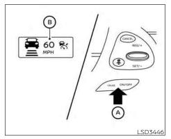
Operating vehicle-to-vehicle distance control mode
