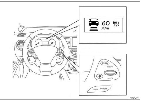
VEHICLE-TO-VEHICLE DISTANCE CONTROL MODE OPERATION The vehicle-to-vehicle distance control mode is designed to maintain a selected distance from the vehicle in front of you and can reduce the speed to match a
