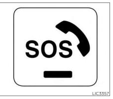
The E-call (SOS) button is used in combination with a NissanConnect® Services subscription to call for assistance in case of an emergency.
