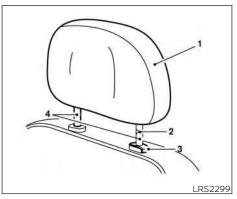
NON-ADJUSTABLE HEAD RESTRAINT/HEADREST COMPONENTS
