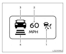
Vehicle-to-vehicle distance control mode display and indicators
