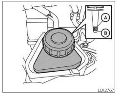
Check the fluid level in the reservoir.
