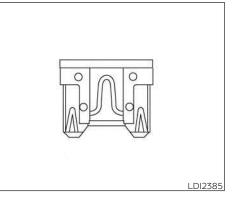
If any electrical equipment does not operate, check for an open fuse.
