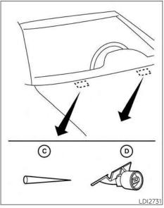
If you wax the surface of the hood, be careful not to let wax get into the washer nozzle O. This may cause clogging or improper windshield-washer operation. If wax gets into the nozzle, remove it with a needle or small pin O.
