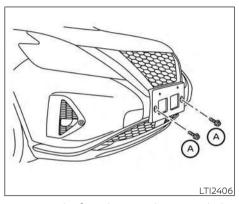
To mount the front license plate, attach the license plate bracket to the plastic finisher at the location marks (small dimples) using the two provided screws O.
