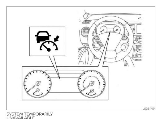
The following are conditions in which the ICC system may be temporarily unavailable. In these instances, the ICC system may not cancel and may not be able to maintain the selected following distance from the vehicle ahead.
