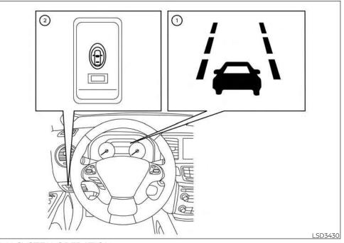
The I-LI system operates above approximately 37 mph (60 km/h). When the vehicle approaches either the left or the right side of the traveling lane, the steering wheel will vibrate and the LDW/I–LI indicator  $\bigcirc$  (orange) on the instrument panel will blink to alert the driver. Then, the I-LI system will automatically apply the brakes for a short period of time to help assist the driver to return the vehicle to the center of the traveling lane.
