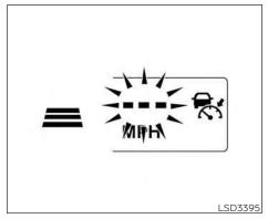
When the SET/- switch is pushed under the following conditions, the system cannot be set and the ICC indicators will blink for approximately 2 seconds:
