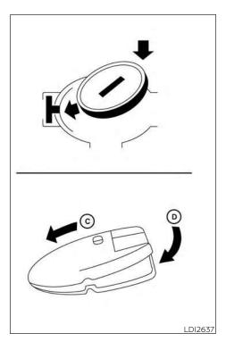
3. Replace the battery with a new one.
