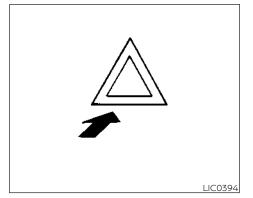
Push the switch on to warn other drivers when you must stop or park under emergency conditions. All turn signal lights flash.
