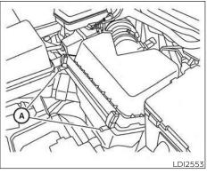
The air cleaner filter should not be cleaned and reused. Replace it according to the maintenance log shown in the "Maintenance and schedules" section of this manual.
