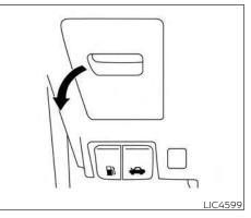
The extended storage switch is pulled out when in transit from the factory to the retailer. It is located in the fuse panel to the left of the steering wheel on the instrument panel. If any electrical equipment does not operate, ensure the extended storage switch is pushed fully in place, as shown.
