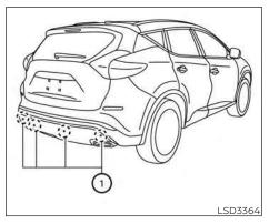
The RAB system detects obstacles behind the vehicle using the parking sensors  $\bigcirc$  located on the rear bumper.
