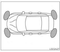
The sonar (parking sensor) system sounds a tone to inform the driver of obstacles near the bumper.
