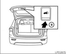
3. Press and hold the power liftgate close switch (B) located on the liftgate for more than 3 seconds or until two beeps are heard.
