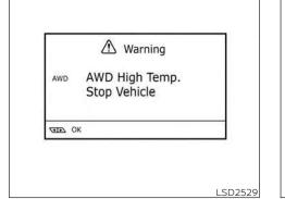
The AWD high temperature message may be displayed while trying to free a stuck vehicle due to increased oil temperature. The driving mode may change to 2-Wheel Drive (2WD). If this message is displayed, stop the vehicle with the engine idling, as soon as it is safe to do so. Then if the message turns off, you can continue driving.
