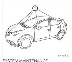
If dirt, rain or snow accumulates on any of the cameras ①, the MOD system may not operate properly. Clean the camera by wiping with a cloth dampened with a diluted mild cleaning agent and then wiping with a dry cloth.
