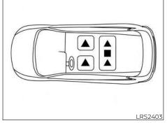
The illustration shows the seating positions equipped with head restraints/headrests.
