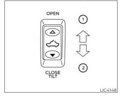
The moonroof will only operate when the ignition switch is placed in the ON position. The moonroof is operational for a period of time, even if the ignition switch is placed in the ACC (if so equipped) or OFF position. If the driver's door or the front passenger's door is opened during this period of time, the power to the moonroof is canceled.
