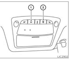
When the ON switch  $\bigcirc$  is pushed, the footwell lights (if so equipped), step lights (if so equipped), map lights and rear personal lights will automatically turn on and stay on for a period of time when:
