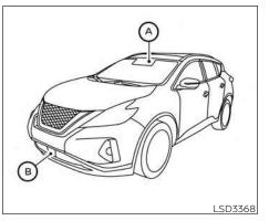
The AEB with Pedestrian Detection system uses a radar sensor located on the front of the vehicle (a) to measure the distance to the vehicle ahead in the same lane. For pedestrians, the AEB with Pedestrian Detection system uses a camera installed behind the windshield (A) in addition to the radar sensor.
