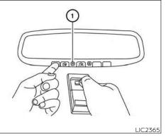
1. Position the end of your hand-held transmitter 1-3 in (2-8 cm) away from the HomeLink® surface, keeping the HomeLink® indicator light ① in view.
