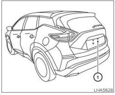
If dirt, rain or snow accumulates on the camera  $\bigcirc$ , the RearView Monitor may not display objects clearly. Clean the camera by wiping it with a cloth dampened with a diluted mild cleaning agent and then wiping it with a dry cloth.
