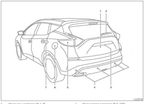
6. Fuel-filler door (P. 3-28) Fuel recommendation (P. 10-4) Fuel-filler cap (P. 3-28)
