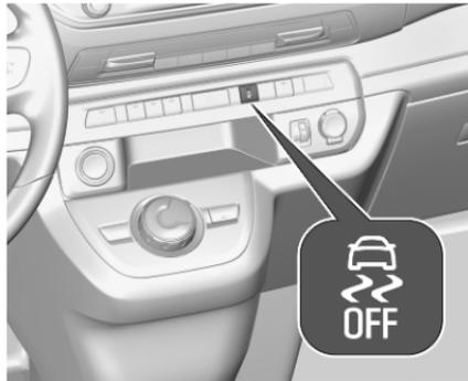
I sistemi ESC e TC possono essere disattivati se necessario: premere
