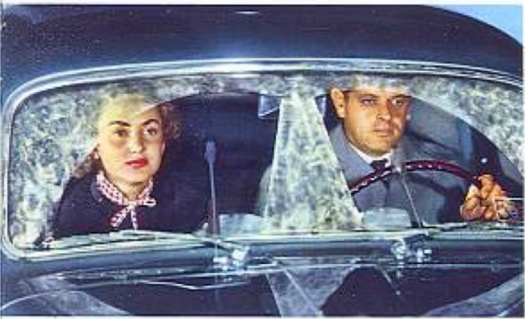
The spray windshield washer cleans the front glass without having to stop the car.
