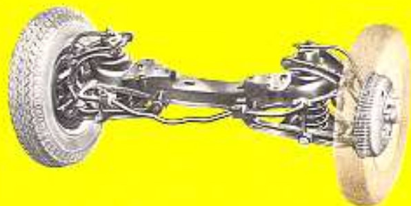
improved suspension, with increased flexibility of front springing; smoother steering as a result of improvements to the steering linkage assembly and to the front axle
