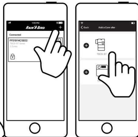
**2.4 EN:** Choose the controller from the list ensuring the serial number matches that printed on the side of the control module.
