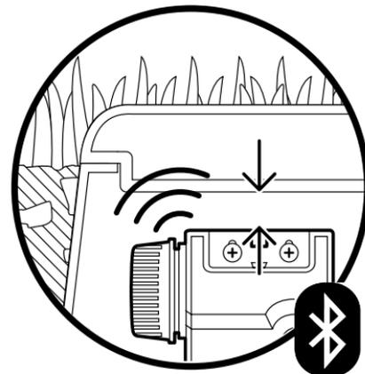
**EN:** To optimize Bluetooth range and signal strength, mount the unit as close to ground surface level as possible.
