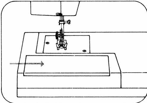
Push the detachable work support onto the machine (guide pin in hole).
