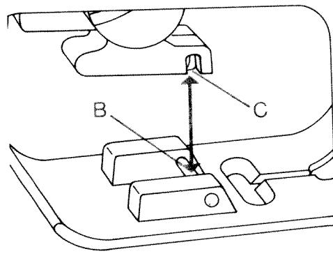
**Attaching the sewing foot:** Lower the presser bar lifter and at the same time reposition the sewing foot so that stud B fits in slots C.
