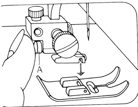
**Changing the sewing foot:** To release the sewing foot, push the red button A.
