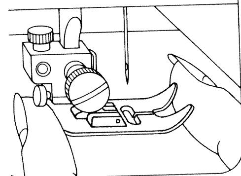
Hole E and screw D are used for **attaching an edge guide**, while screw F is the sewing foot holder screw.
