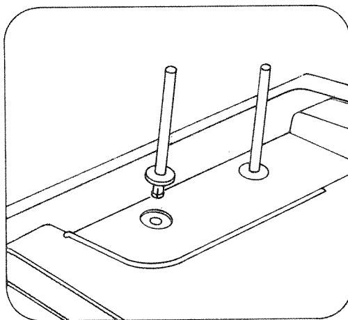
**Inserting the spool pins:**
