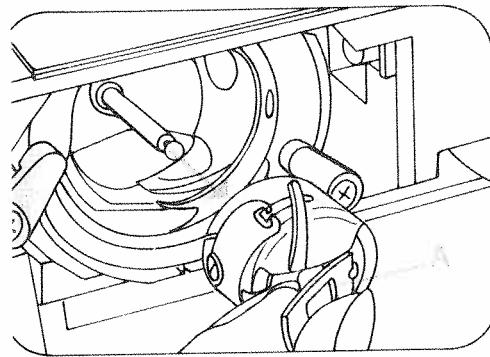
Raise latch A and pull out the bobbin case.
