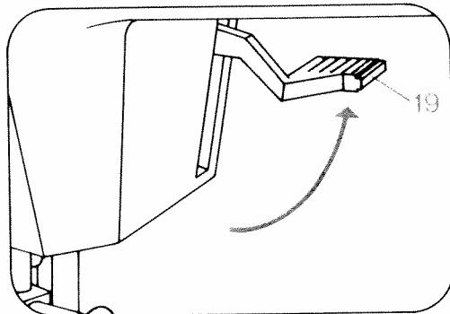
Raise presser bar lifter 19. Remove the fabric by pulling it towards the back.
