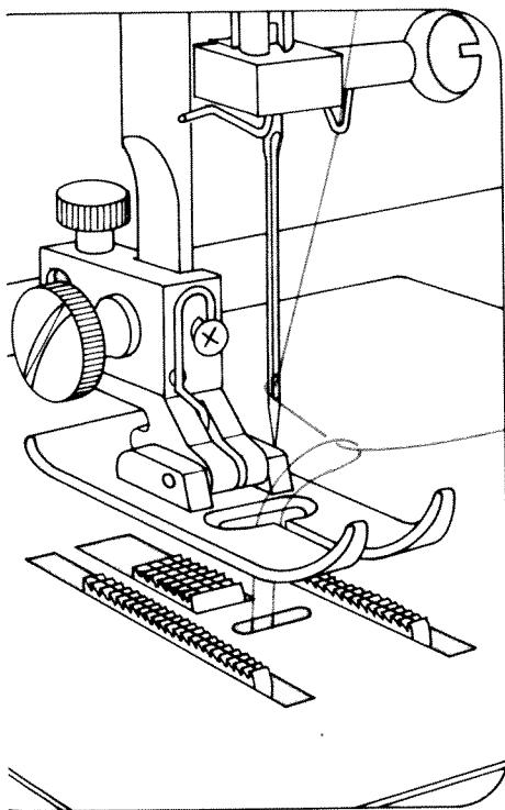
Drawing up the bobbin thread: Hold the needle thread taut. Turn the hand wheel towards you and sew a stitch until both needle and take-up lever are up. Pull out the bobbin thread by means of the needle thread.
