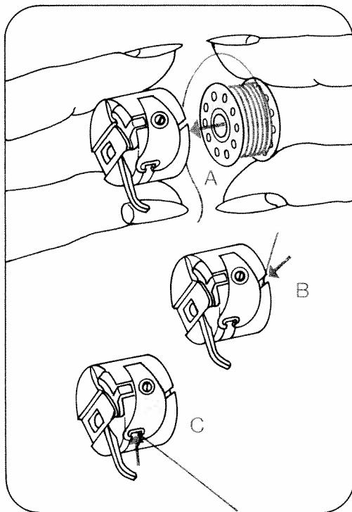
**Inserting the bobbin:** With thread hanging down at back (A), pull it into slot B, under the spring and out of slot C.
