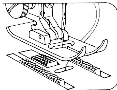
Place both threads towards the right under the sewing foot.
