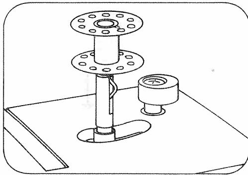
Place the bobbin on winder spindle 5.
