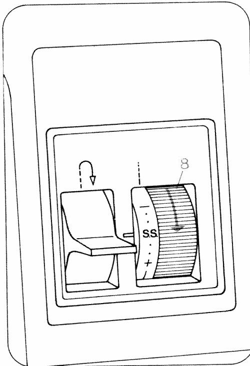
For **sewing stretch stitches**, set the stitch length control a "S. S." Depending on the type of fabric, the stretch stitches can be lengthened by turning the control towards "+" or shortened by turning it towards "-".
