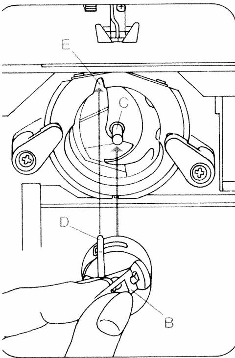
**Inserting the bobbin case:** Open latch B and push the bobbin case onto pin C until it snaps in place. Bobbin case finger D must fit into cutout E.
