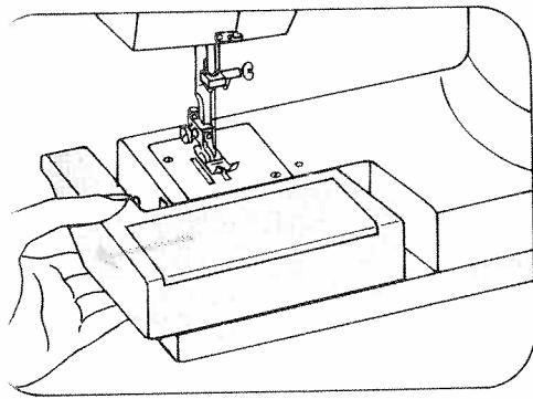
**Bobbin winding preparations:** Reach under work support 9 and pull it out towards the left.
