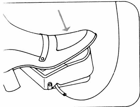
**Operating the foot control:** The farther you press the pedal down the faster the machine runs.
