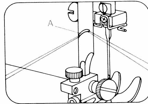
**Thread cutter A:** Draw the threads into the slot and pull them downwards.
