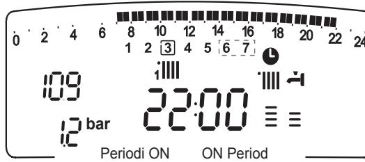
Turn the CH knob
