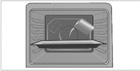
3. Set the oven to easy steam cleaning mode and run at 100°C for 25 minutes.
