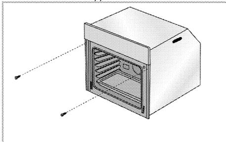
Secure the oven with 2 screws as illustrated.
