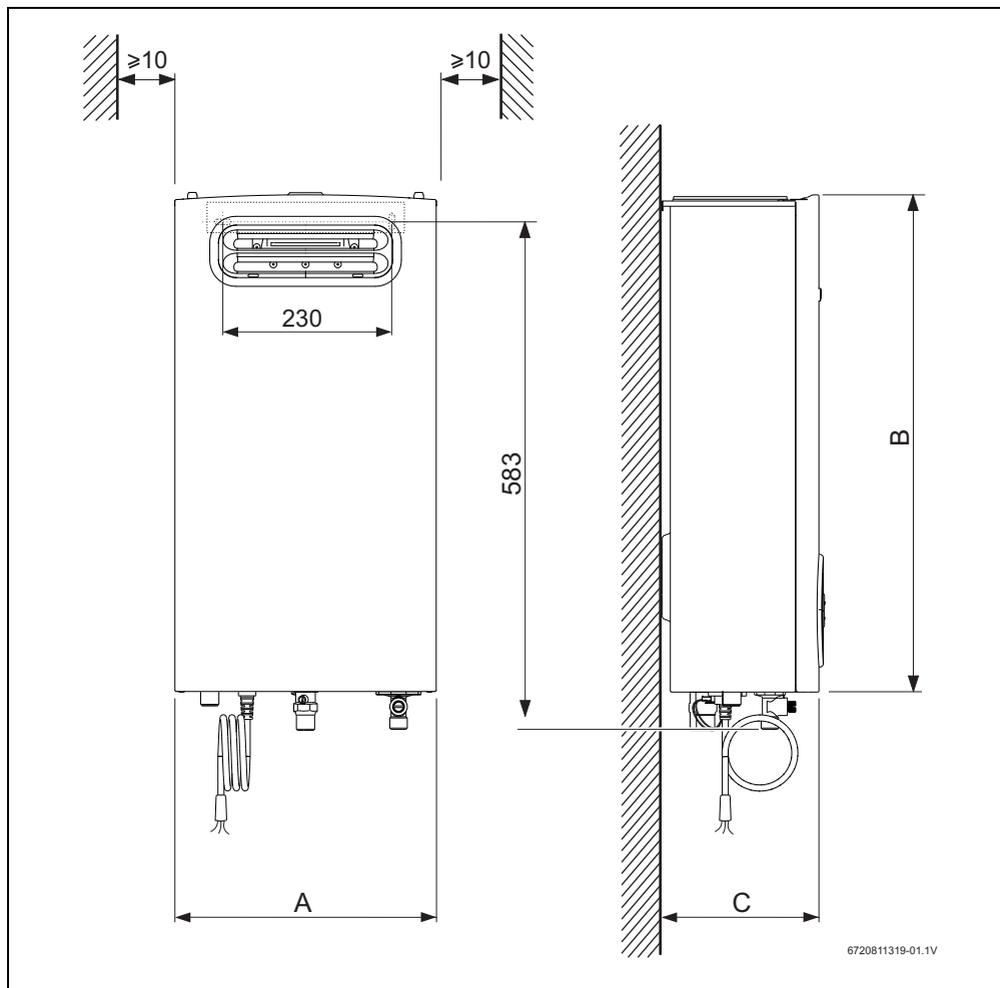
Fig. 1 Dimensioni (in mm)
