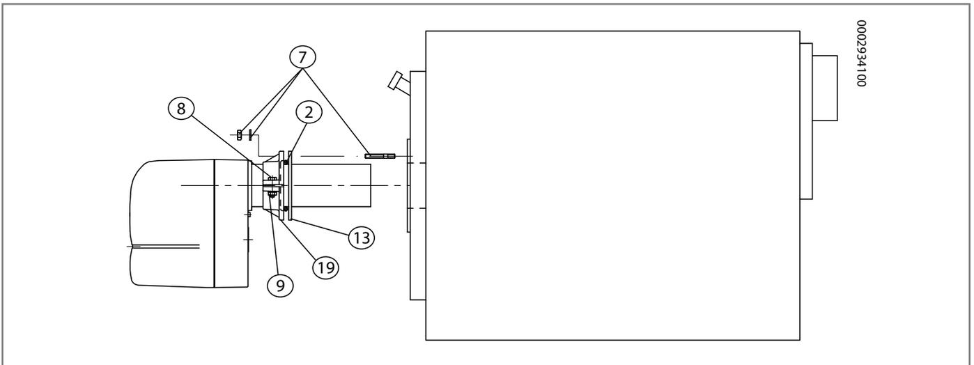
The DUNGS gas valve mod. MB... valve incorporates a filter and a gas pressure stabilizer, therefore, only a cut-off valve and an anti-vibration joint have to be fitted onto the gas pipeline.
