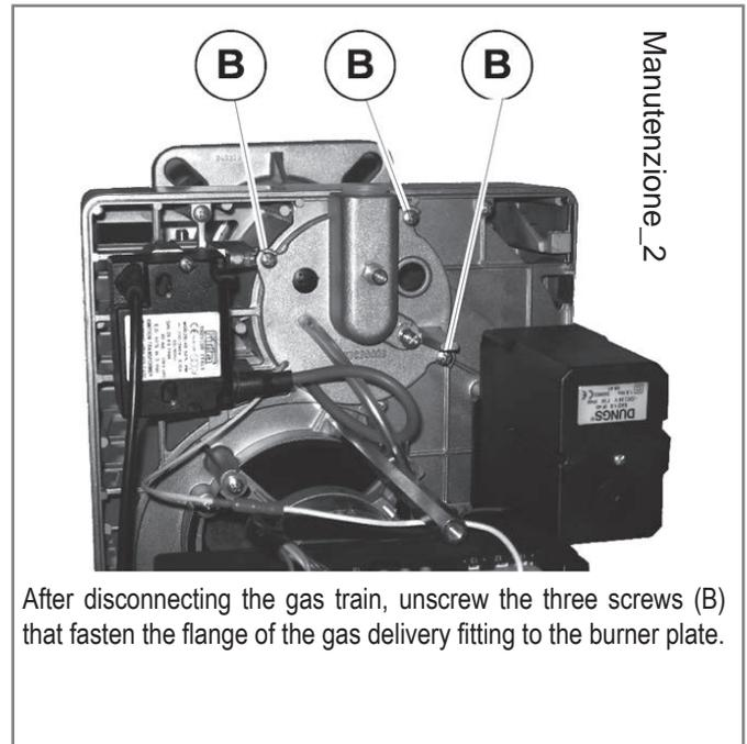
After disconnecting the gas train, unscrew the three screws (B) that fasten the flange of the gas delivery fitting to the burner plate.
