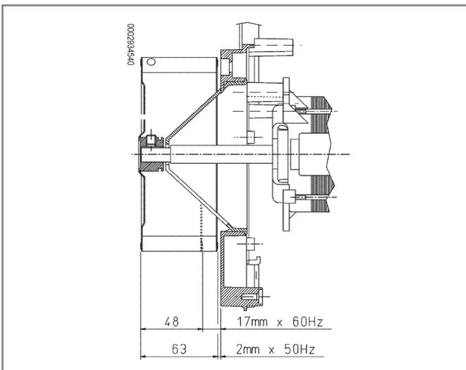
During fan assembly, check that the dimension indicated is respected.
