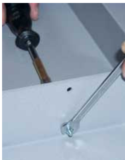
C Couple and secure the right and left side panels, following the summary table at point "B".
