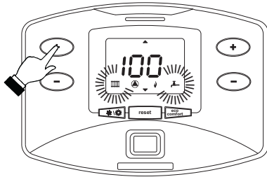
fig. 30 - TEST mode (heating power = 100%)
