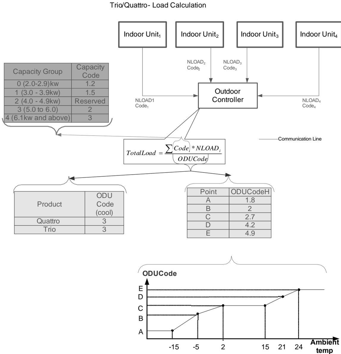
Compressor speed will be set between the minimum speed and the max speed according to the ODU NLOAD
