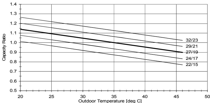
**5.7.3 Heating Capacity Factors - Unit A,B,C or D**
