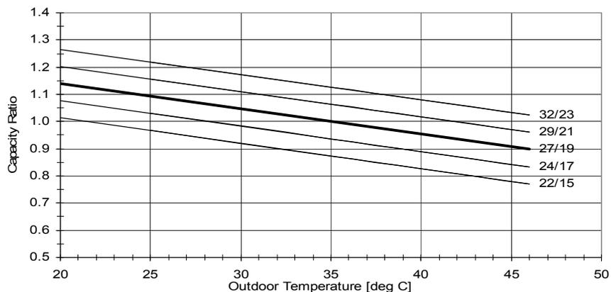
**5.6.3 Heating Capacity Factors - Unit A,B,C or D**
