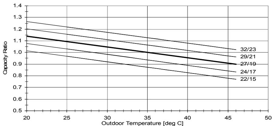
**5.3.3 Heating Capacity Factors - Unit A,B,C or D**
