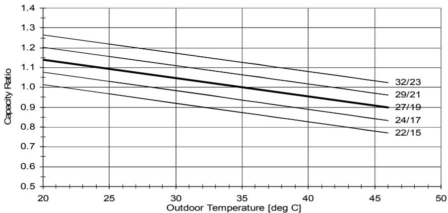
**5.4.3 Heating Capacity Factors - Unit A,B,C or D**
