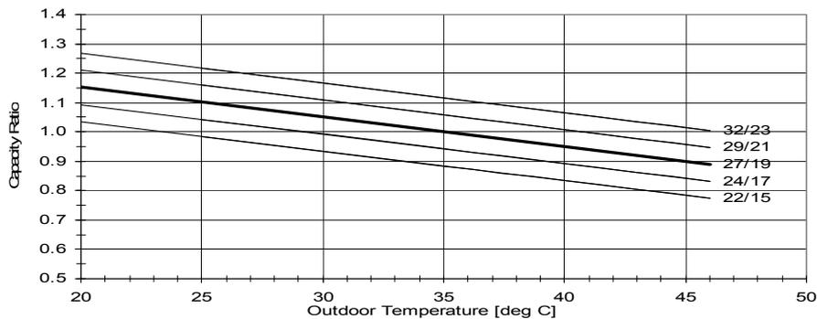
**5.5.3 Heating Capacity Factors - Unit D**
