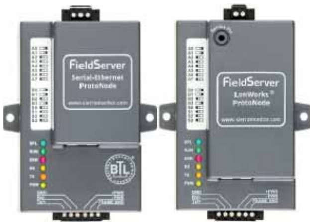
IS to Bacnet / Lonworks
