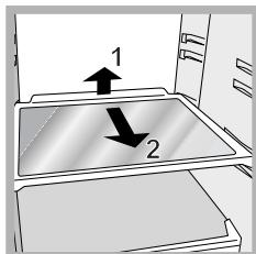
**SHELVES**: the shelves are removable and their height may be adjusted thanks to special rails (see diagram), allowing easy storage of large containers and bulky food. The height may be adjusted without removing the shelf completely.
