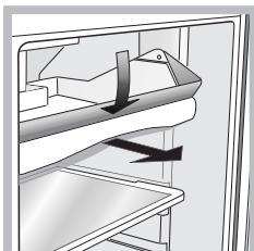
**FRESH BOX\***: for fresh meat and fish. Due to the compartment's low temperature (the coldest in the refrigerator) and to the clear door that provides protection against oxidation and blackening, food can be stored for even up to one week. It can also be used for "cold meals."
