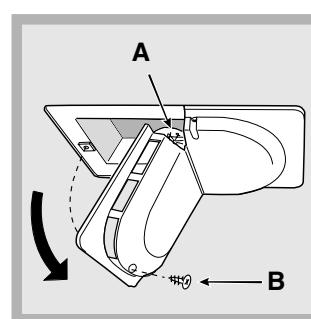
Access the light bulb (A) by unscrewing the fixing screw (B) which is located at the back of the lampcover, as shown (see diagram). Replace it with a similar light bulb, the power of which should not exceed 15W.
