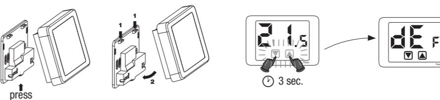
Unhook and re-hook the thermostat from the base (battery models) or remove and restore power (230V models). Press the keys for at least 3 seconds during the flashing.
