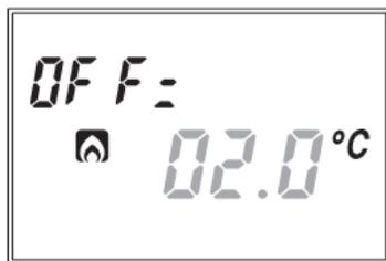
It is also possible to disable the antifreeze function holding the "▼" key until field **(16)** displays the symbol "----". In this case, when the chronothermostat is off, no regulation is executed.
