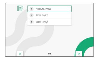
Only for video door configured powered in **Low rise block** and **High rise block** modes, access to the video door phone book is permitted to one device at a time, for a maximum of 5 minutes. If a user tries to access the book when it is already used on another device, the video door phone will emit a dissuasion tone (4 beeps) indicating that the address book cannot be displayed at the moment.
