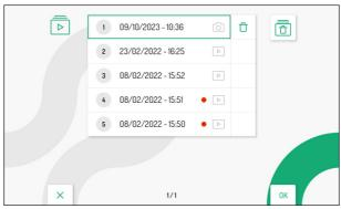
Press the  $\nabla$  and  $\triangle$  keys to select the video clip or screenshot, then press the  $\bigcirc$  key to viewing.
