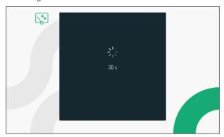
The keys are inhibited for 30 seconds, after which the video door phone resumes its normal operation. Once the "Clean Screen" function is activated, you cannot turn it off in advance.
